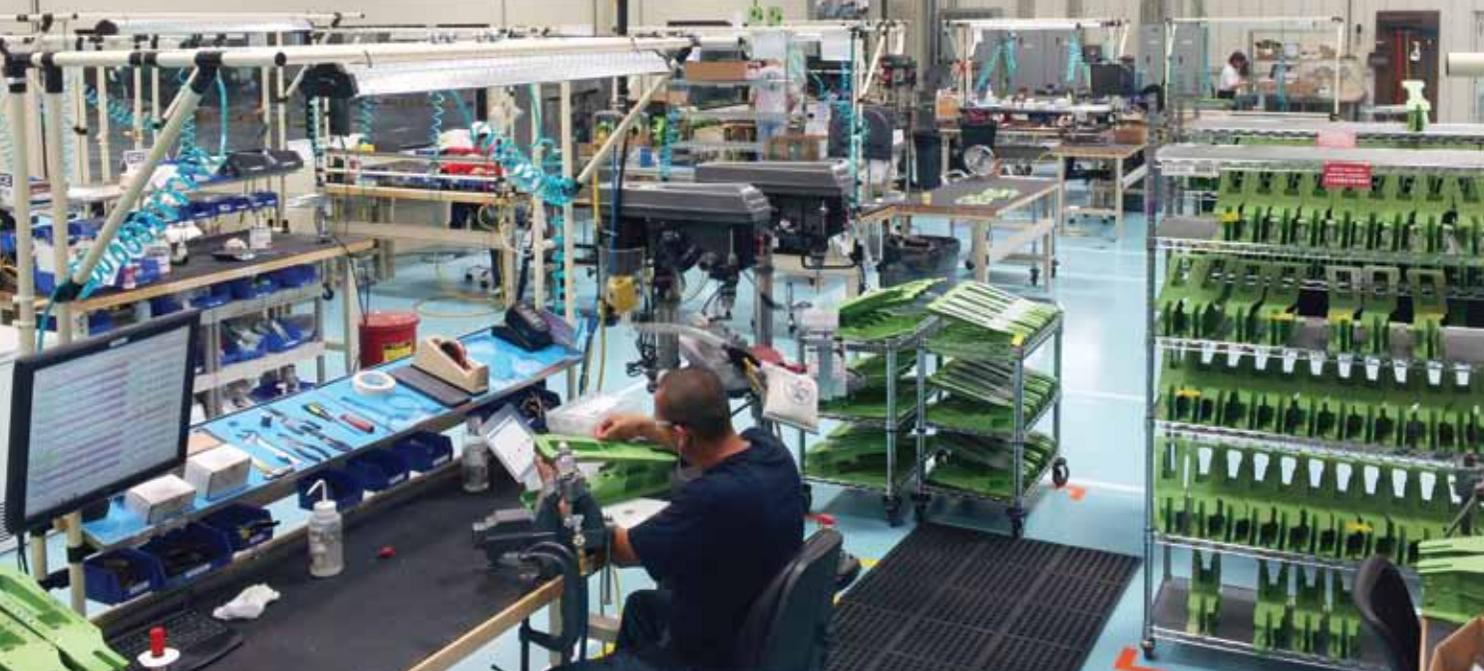
*Aircraft structural components are assembled in lean assembly cells.*
