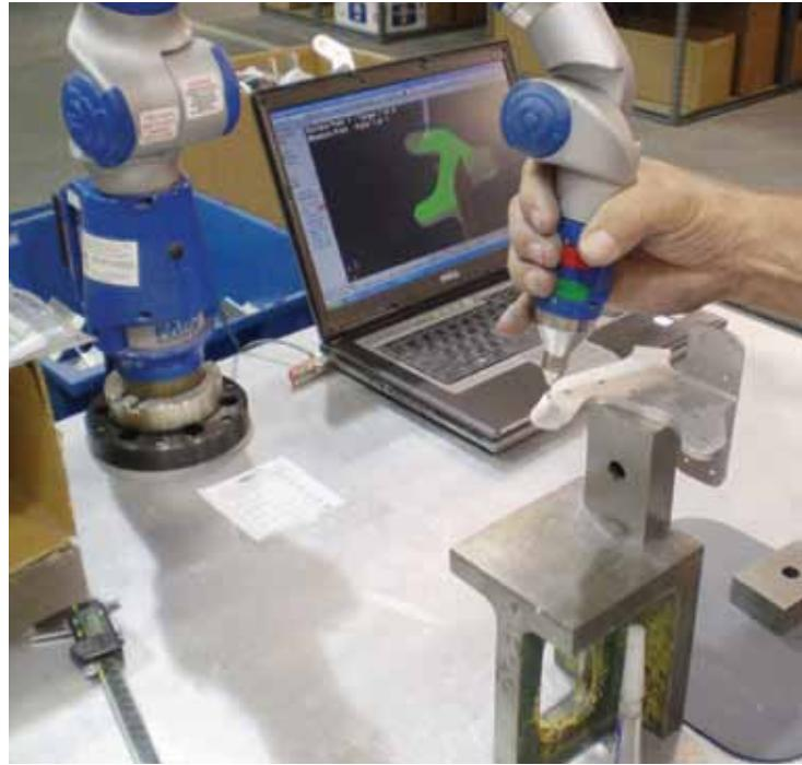
**Parts are inspected against a solid model on the manufacturing floor.**
