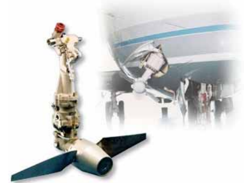
Ram Air Turbine
